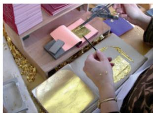
The final beating process requires roughly 5,000 to 7,000 hammer strikes and can take anywhere between two and a half and six hours to accomplish. The special hammers used by gold beaters weigh between 2 and 12.5 kg. The process of inserting and quartering is carried out by the gold adjusters.
